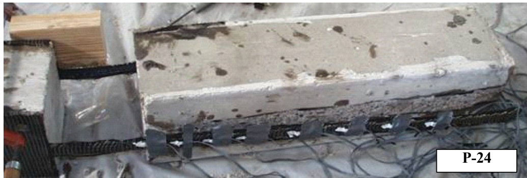
Figure 2.52 Failure Anchorage Specimens (P Series)
